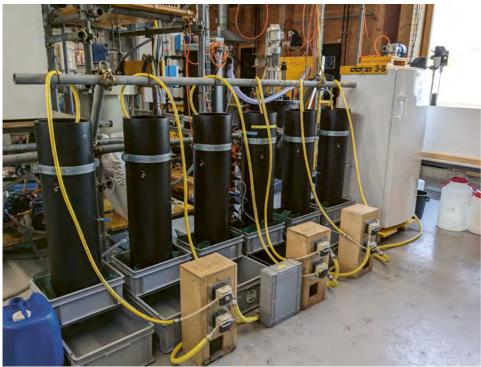
Photo: To better understand the mechanisms effecting the nitrogen cycle throughout vermifiltration, the six lab-scale reactors seen in this photo have been installed at Eawag and tests are ongoing. Three of the six filters are currently receiving blackwater (flush water, urine, faeces and toilet paper) and the other three are receiving brown water (flush water, faeces and toilet paper).
